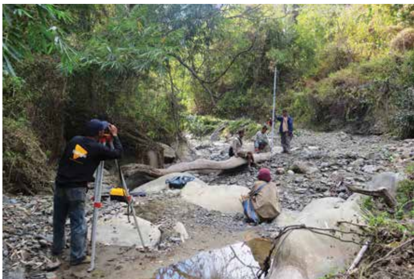
Burma – Topographical survey intended to quantify the building materials for an irrigation work. Survey carried out by the communities with the technical support of Triangle G H teams - Photo: Thang Kip Lian / Triangle G H
